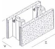
**Figure 2.** Interlocking masonry unit.
