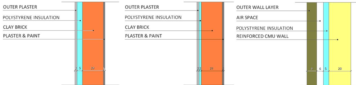
**Figure 7.** Types of walls to be compared. Left traditional wall with 5cm. insulation, middle traditional wall with 2 cm. insulation, right NP 12’s wall system.
